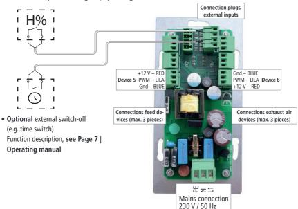
A data line is recommended (e.g.  $2 \times 2 \times 0.6$  (z. B. J-Y(ST)Y)) for the connection of external control inputs (potential-free contacts).
