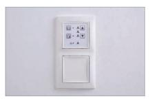
The **controller** is designed for installation in a device double socket. It can be used to control up to six **AirUnits**. The **controller** is to be connected as stationary equipment with permanently laid lines. Electrical connection diagram, **see page 10**.
