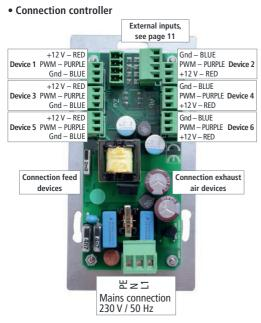
The connection of several devices occurs arranged in pairs at the plug connectors **device 1 - device 2**, **device 3 - device 4**, **device 5 - device 6**; in paired operation one device of a device pair operates in feed mode, the second assigned device in exhaust air mode The air flow direction of both devices is alternated at intervals.
