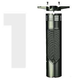
Remove the table leg from the box and place it as shown in the picture. Remove the transport protection by loosening the two screws. Then remove the top brackets and install it with two screws and washers
