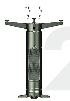
Place the table leg standing on the top bracket, so that the top bracket is facing the ground/ floor. Remove the transport protection by loosening the the two screws. Route the cord through the leg and pull it up so that it fits the table leg. Make sure the cord is positioned correctly, so that it is located directly next to the hole in the foot. Fasten the foot with the two screws.
